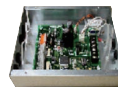
Relay Interface BMS-IFWH5E For Energy Monitoring to connect power meter Relay Interface BMS-IFDD03E To connect external digital input/output
