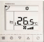
Wired Remote Controller RBC-ASC11E • Compact size H86mm x W86mm x D16mm • Stylish design with big screen and backlight • Schedule timer (off only) • Operation mode, error code display • Temperature control in steps of 0.5°C
